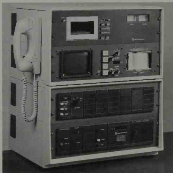
Figure 12.17 Emergency medical care system. (a) Portable transmitter unit. (b) Transmitter unit in use. (c) Hospital console. (Courtesy of Motorola Communications and Electronics Inc., Schaumburg, IL.)
