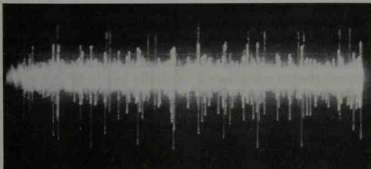
Figure 10.9. Gross measurement of multiple unit neuronal discharge. (Full width covers time span of 500 msec. Maximum peak-to-peak amplitude is approximately 145 microvolts.) (Courtesy of Neuropsychology Research Laboratory, Veterans Administration Hospital, Sepulveda, CA.)
