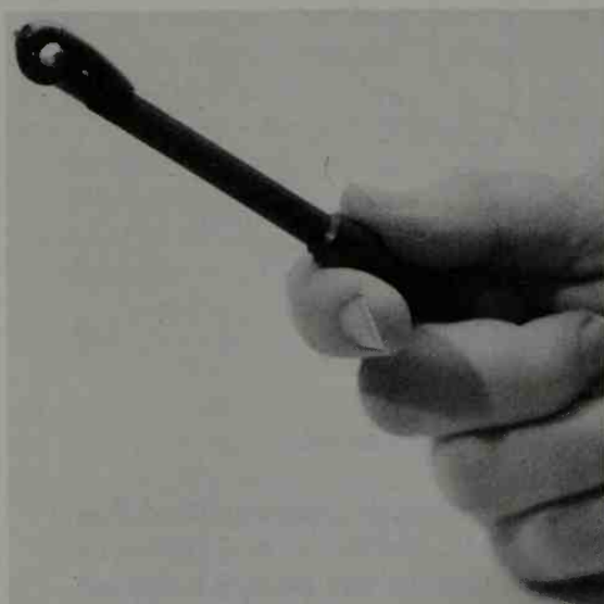
Figure 6.31. Blood flow probe—clip-on type for use during surgery. (Courtesy of Biotronex, Silver Springs, MD.)
