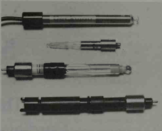
Figure 4.20. Specific ion electrodes with pH glass electrode. (a) Sodium ion electrode; (b) cationic electrode; (c) pH glass electrode; (d) ammonia electrode. (Courtesy Beckman Instruments, Inc., Fullerton, CA.)
