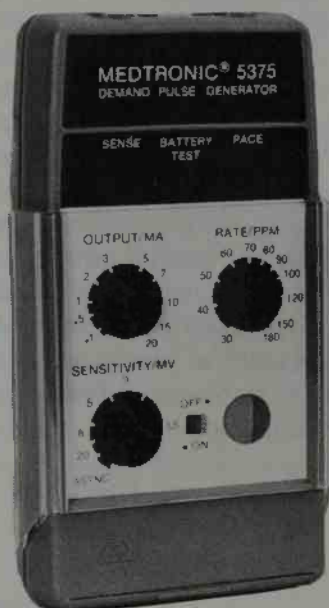
Figure 7.18. Portable external pacemaker, strapped on arm. (Courtesy of Medtronic, Inc., Minneapolis, MN.)
