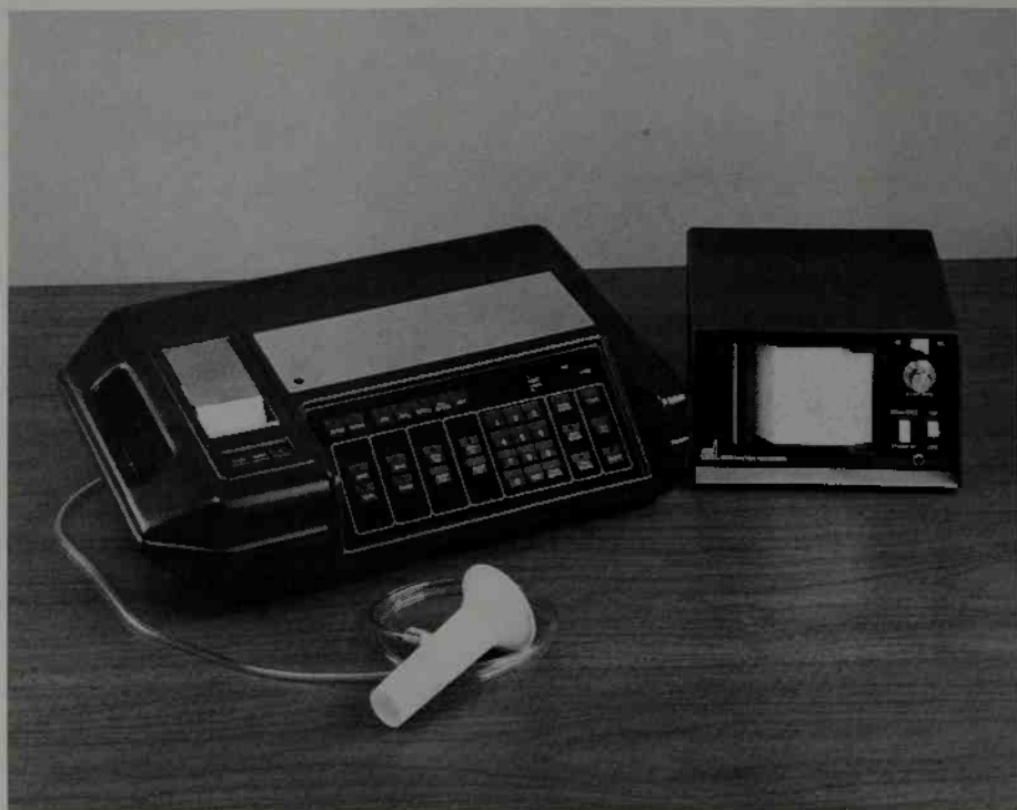
Figure 8.6. Electronic spirometer with digital readout, printed tape, and computer interface capabilities. (Courtesy of Life Support Equipment Co., Woburn, MA.)
