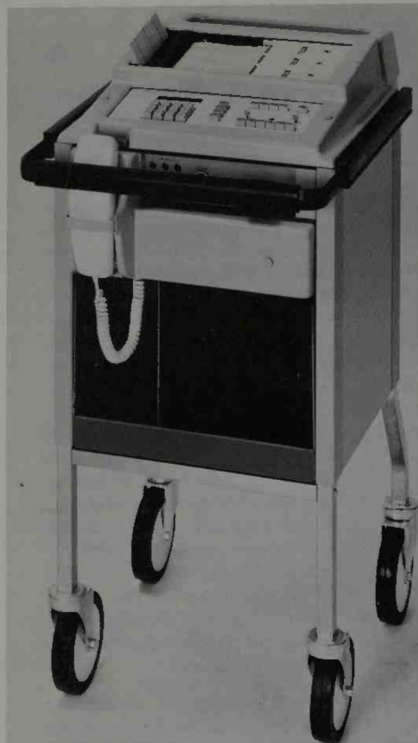
Figure 6.10. Automatic three-channel ECG recorder with keyboard for entering patient data and telephone coupler to send ECG and data to a remote computer via telephone lines. (Courtesy of Hewlett-Packard Co., MA.)
