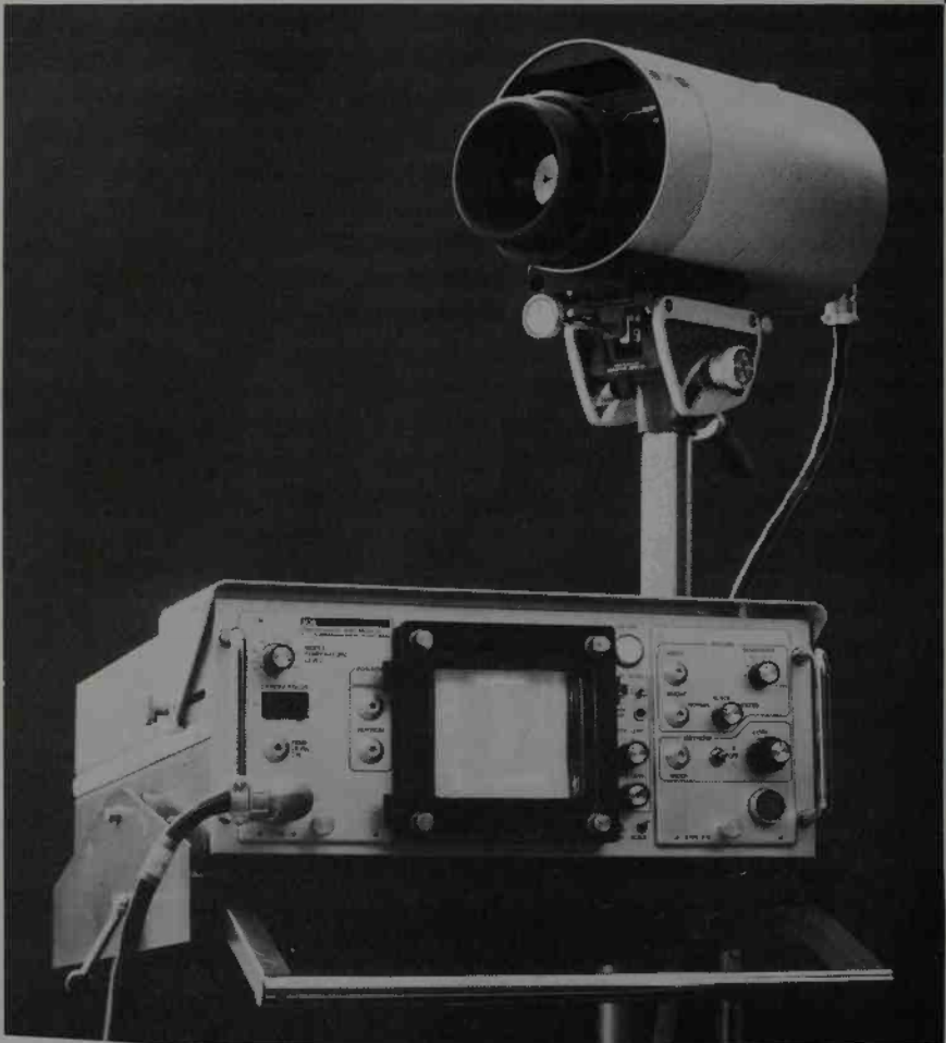
Figure 9.6. Thermovision system: (a) Thermovision 680 Medical, camera and display unit; (b) Thermovision 680 Medical with accessories. (Courtesy of AGA Infrared Systems AB, Sweden.)
